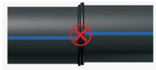
Dry-welding: welding rings are too narrow, usually due to low temperature or shortage of pressure
