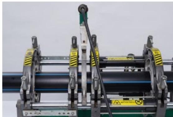
4. The heated pipe ends are then retracted and the heater plate removed as soon as possible (t3: no contact pressure).
