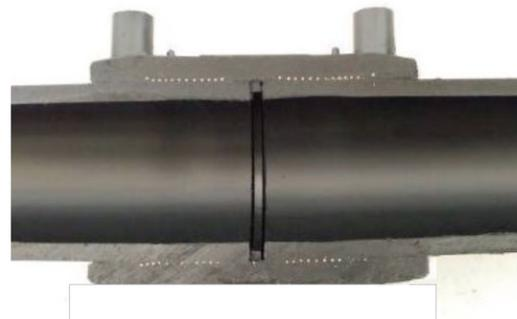
Figure 8.2.3.A Typical Electrofusion
