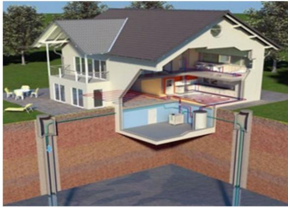
VASEN PE piping system for GSHP(Ground Source Heat Pump) application
