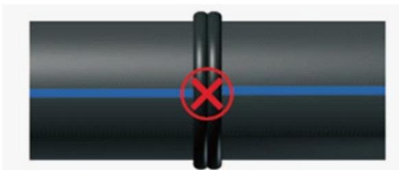
Unfitness butt fusion: the two pipes are not in alignment
